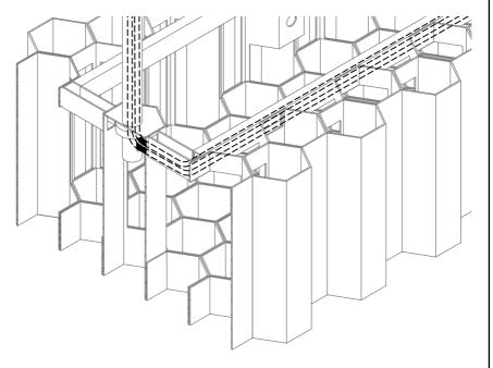
Pass carefully the wires through the holes
